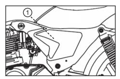
The air filter (1) should be replaced according to the maintenance schedule.
