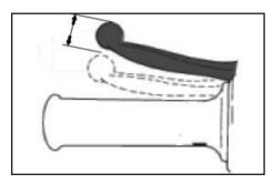
Periodically check the brake lever free play and, if necessary, adjust it as follows.
