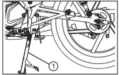
The main stand (1) is located on the left side of the vehicle. Release the main stand by using your feet to step on the bracket of side stand to up-right position to stand the vehicle.
