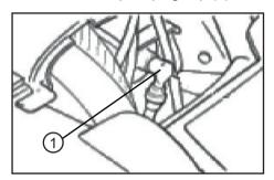
3. Remove the spark plug as shown, with the spark plug wrench (2) included in the owner's tool kit.
