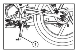
The side stand (1) is located on the left side of the vehicle. Release the sidestand by using your feet to step on the
