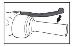
The front brake lever is located on the right handlebar grip. To apply the front brake, pull this lever toward the handlebar grip.
