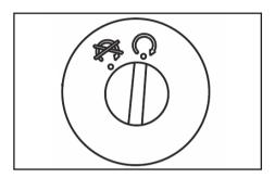
The main switch controls the ignition and lighting systems, and also used to lock the steering. The various positions are described as below.
