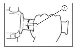
The throttle cable free play (1) should measure  $1.5 \sim 3.5$  mm at the throttle grip.
