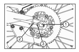
Tightening torque of the collor nut (1): 70 Nm
