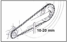
If the chain tension is too great, parts within the secondary power trasmission (chain, chain sprockets transmission and rear wheel bearings) will be subjected to unnecessary stress resulting in early wear and even chain breakage. Too much slack in the chain, on the other hand, can result chain jumping off the chain wheels. If this happens the chain could also block the rear wheel or damage the engine. In either case the operator is likely to lose control of the vehicle.
