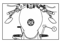
The brake pedal (1) is located on the right-hand side of the vehicle and operates the rear brake. Familiarise yourself with how it works before you ride the vehicle on public roads. Novices and returning riders are recommended to take a riding techniques course.
