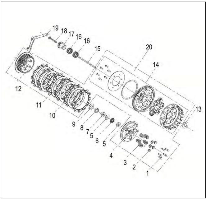
1 Bolt 2 Spring washer 3 Clutch spring 4 Pressure plate 5 Bearing washer 6 Surface needle bearing 7 Clutch separation shaft sleeve 8 Jam nut 9 Locking washer 10 Friction plate assembly 11 Driven plate 12 Clutch driven hub 13 Thrust washer 14 Clutch driving drum assembly 15 Internal separation mandrill 16 Needle roller bearing 17 Bushing 18 Internal separation mandril | 19 Separation drag bar weld assembly 20 Clutch assembly
