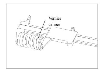
Measure the outer diameter of the valve stem. Allowable limit: Intake  $\Phi4.455 \text{ mm}$
