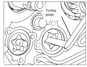
Check the clearance between the outer rotor and pump body
