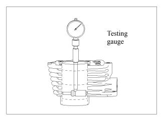
Measure the roundness of cylinder inner wall (internal diameter difference between X direction and Y direction).
