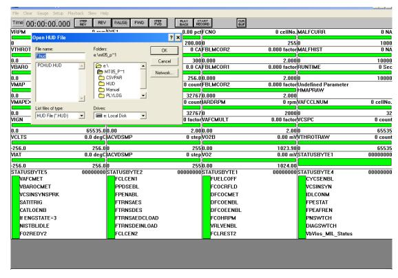
(4) Select "Parameter File" under the "Setup"; click MT05common.par file; select "Comm protocol" under the "Setup"; select "Keyword2000," and then click OK, at the same time Device Code selects 17.
