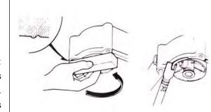
Installation of rubber hose (fuel, vacuum, or coolant): insert its end into bottom of connector so that there is enough room for the hose clamp to grip the connector. Install the rubber or plastic dust cover back to its originally designed position
