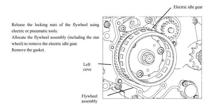
Disassemble the right cover of the crankcase
