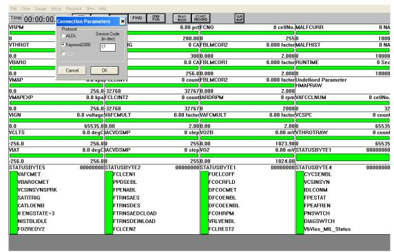
(5) If the software interface cannot display real-time communication data in the case of power, it needs to continue the following work, under "Setup" check whether there is problem with COM port connection settings, and the usual settings are COM Port: 4, the Baud Rate: 10400; do not Select the DTR High at the startup.
