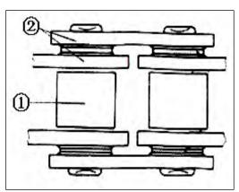
Lubricate drive chain. Buy it from store Check drive chain. Wash, lubricate and replace it if it is hard.
