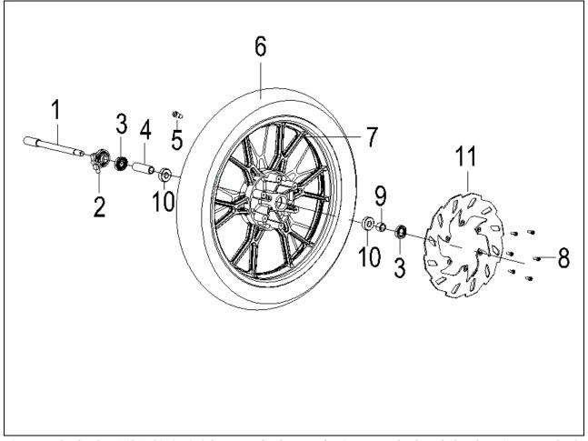
1 Front wheel axleM14\*1.5\*219 2 Odometer wheel gear units 3 Front wheel sealed units 4 Front wheel middle shaft sleeve 5 Cycle valve6 vacuum tyre 100/80-17 7 Front wheel ring 8 Liquid brake plate erection bolt
