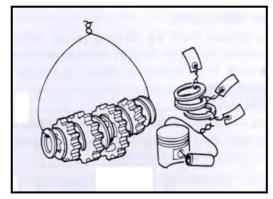
Pay special attention to the key fitting position before disassembly. The components that are not used any more
