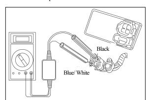
vehicle and remove connector of alternator. Trigger (blue/white) is connected with a shunt.
