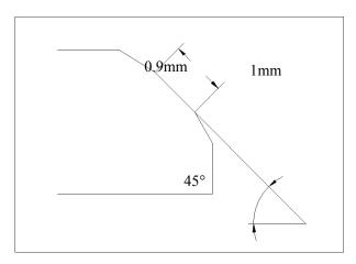
If contacted place is the higher part of valve, please use a  $32^{\circ}$  angle plain milling cutter to lower the valve race. If contacted place is the lower part of valve, please use a  $60^{\circ}$  angle internal milling cutter to raise the valve race.
