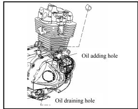
Check if there is engine oil leakage. Start the engine and run the engine on idle for a few minutes. Check engine oil level again.
