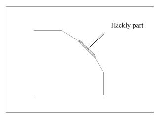
Remove 1/4 of external edge of valve race with a 30° angle milling cutter.
