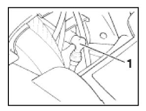
Disassemble spark plug with spark plug sleeve.
