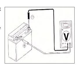
Voltmeter shall be used for charging inspection.
