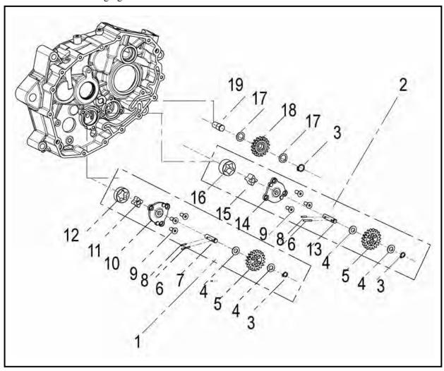
1 Oil suction pump assembly 2 Oil pressure pump assembly 3 Retaining ring 4 Gasket 5 Oil pump gear 6 Fixed pin 7 Oil suction pump shaft 8 Pin 9 Bolt M6x16 10 Oil pump cover 11 Inner rotor 12 Outer rotor 13 Oil pressure pump shaft 14 Oil pump cover 15 Inner rotor 16 Outer rotor 17 Gasket 18 Oil pump transition gear 19 Transition gear shaft
