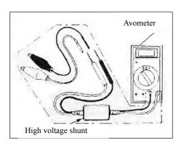
Connect a high-voltage shunt or an ammeter with input impedance higher than  $10M\Omega$  10CV to the multimeter.
