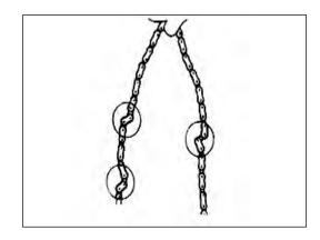
Check drive chain and driven chain wheel. Replace chain wheel when 1/4 gear teeth are worn. Replace it when gear teeth is bending.
