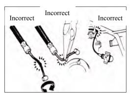
Plastic parts may age and deteriorate, which are apt to be damaged by solvent or oil. Check before re-installation and replace if necessary.
