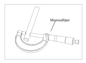
Measure the inner diameter of the shifting fork hole. Allowable limit: 10.05mm.
