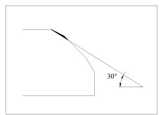
Remove 1/4 of bottom of valve race with a  $70^{\circ}$  angle milling cutter.
