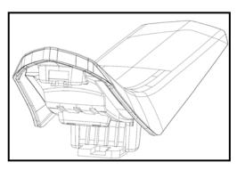
Disassemble backplate of the right fuel tank Disassemble right knee board.
