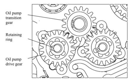
Remove the fixed pin, the screw and the pup cover, and disassemble the oil pump;
