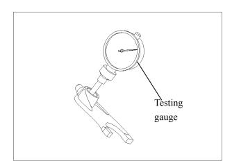
Measure the thickness of the shifting fork. Allowable limit: 4.6mm
