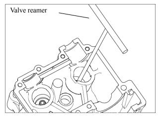
Remove carbon deposited in combustion chamber and valve and clean thoroughly intake and exhaust valves.
