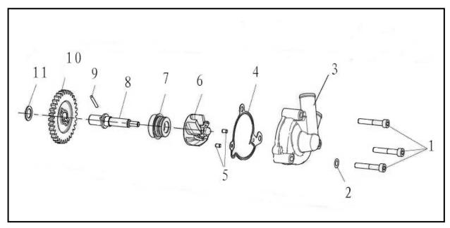
1 Hexagon socket cylinder bolt 2 Gasket 6 3 Water pump cover 4 Water cover seal gasket 5 Pin 6 Impeller 7 Water seal assembly 8 Water pump shaft 9 Pin3\*22 10 Water pump gear 11 Gasket
