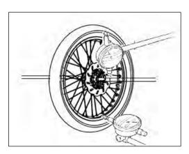
When rear wheel shimmy exceeds service limit, rear wheel bearing is loosened, which results in wobbly rear wheel. Check and replace rear wheel bearing.
