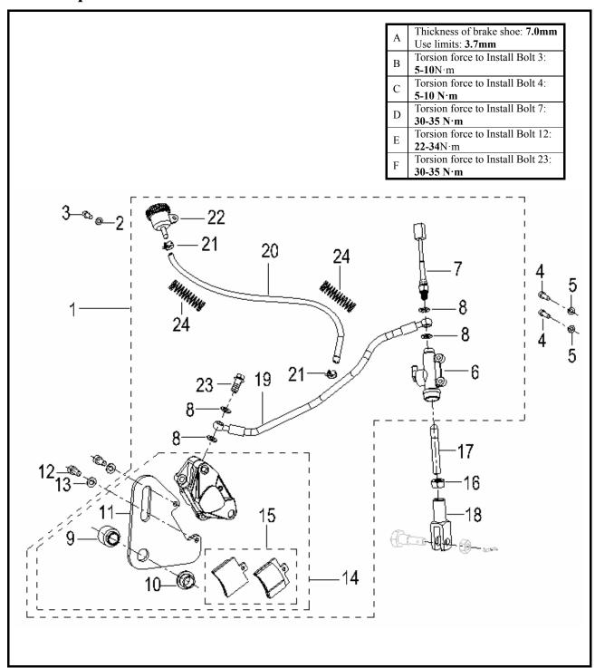
Rear liquid brake block units Gasket 6 Inner hexagon screw M6\*16 Inner hexagon screw M6\*16 Gasket 6 Oil pump assembly Brake switch assembly Seal ring Lining I Lining II Connecting plate Inner hexagon screw M8\*20 Gasket 8 Brake cylinder B Friction plate units Draw bar Nut M6 Draw handle Brake hose unit Oil tube (21) Hoop (22) Oil cup units (23) Hexagon flange head tapping screw (24) Protecting spring
