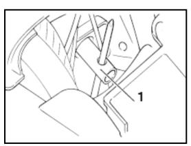
Check the burning, pollution and carbon deposit of spark plug.
