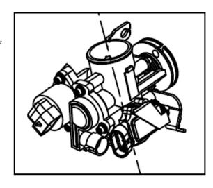
If idle speed RPM is unsteady, or idle speed is not smooth when gently raise engine speed, adjust idle speed adjusting screw again.
