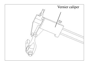
Measure the outer diameter of gearshift drum. Allowable limit:  $41.75 mm_{\circ}$
