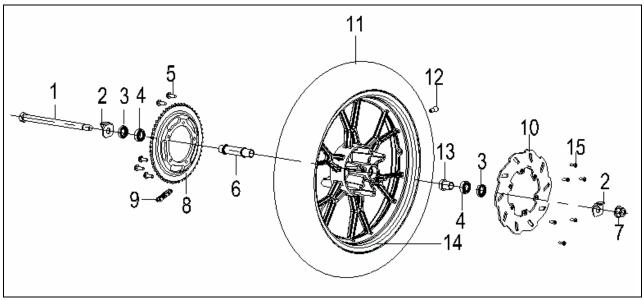
1. Rear axle 2. Rear wheel plate pinch 3. front wheel oil seal assembly 4. Rolling bearing 6003-2RS 5. Chain erection bolt M8\*22 6. Rear wheel central axle sleeve units 7. Self-locking nutM16\*1.5 8. Chain wheel 9. Chain 428HG-1\*132 10. Rear brake disc 11. Vacuum tyre 130/80-17 12 . Cycle valve 13. Rear wheel left axle sleeve 14. Rear wheel ring 15. Liquid brake plate erection bolt
