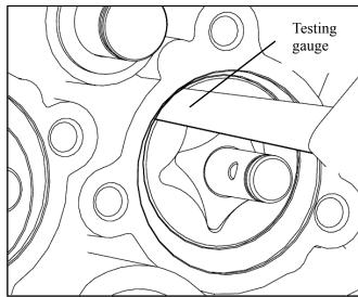
Check the clearance between the rotor ends Allowable limit: 0.15 mm
