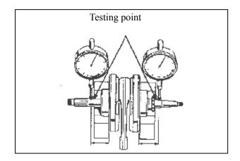
Check whether there is abnormal sound or loose for the revolution of the crankshaft bearing. If any, replace the crankshaft assembly.
