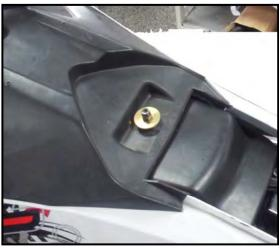
Disassemble air filter cover; fix bolts; take down the cover. Disassemble bolts; take down air filter. Disassemble filter sponge from air filter.
