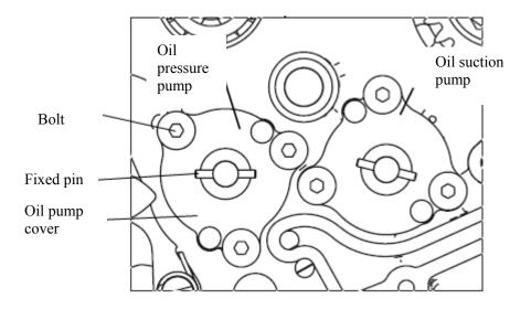
Check the radial clearance between the inner and outer rotor
