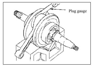
Measure the clearance in the X-Y direction of the big ends of connecting rod.
