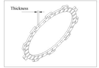
Check the flatness of the driven friction plate with the plug gauge.
