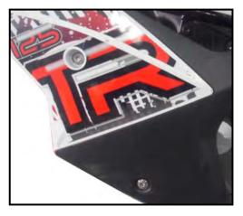
Disassemble backplate of the left fuel tank Disassemble left knee board.
