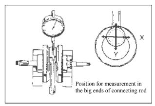
Measure the jumping of the crankshaft. Allowable limit: 0.03 mm.
